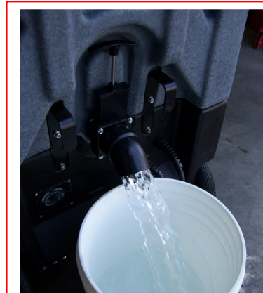
Vacuum acid solution out of Solution Tank
