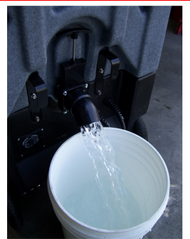
Draining the Recovery Tank
